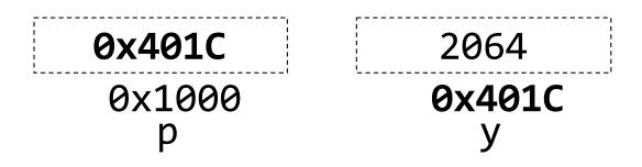
ints occupy 4 bytes. 0x401C is the address of the first byte<sup>\*</sup>:
